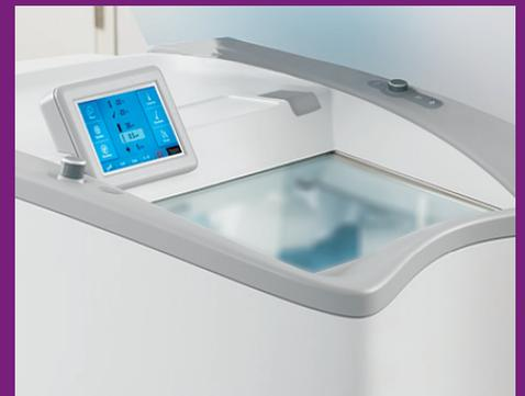
Optional cold disinfection system for NX50 and NX70 cryostats
