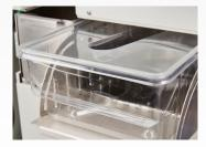
Epredia Paraffin Kit with Waste Wax Drawer are designed for easy and safe disposal – no spilling of hot wax, no burns, just remove the full single use waste wax drawer and discard the entire drawer.
